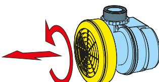
direction of screwing the filter free
