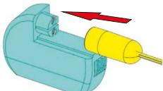
arrows indicate direction of connecting / disconnecting the charger connector
