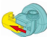
pull the battery from its rails in the direction of arrow
