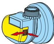
release the position lock and push the battery in the direction of arrow at the same time
