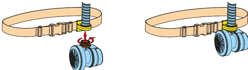
REPLACING THE FILTER [A1]
