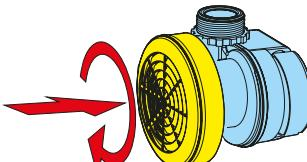
direction of screwing the filter to place
